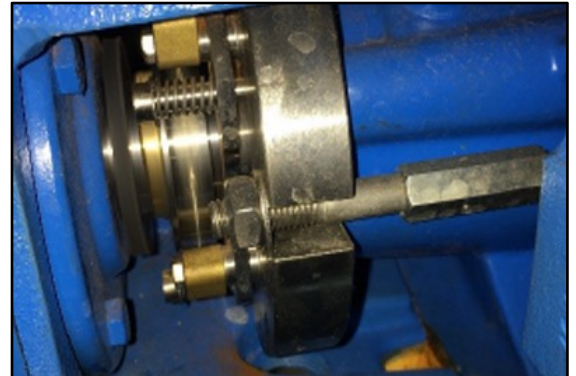
Chesterton 170 Slurry Seal running successfully.
